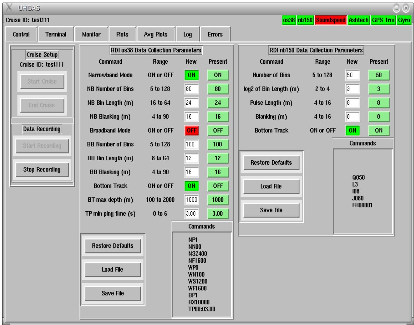
Figure 1: UHDAS control tab, showing control and setup parameters for two ADCPs: an OS38, and the original Narrowband 150. (VmDas cannot be used with this early instrument from RDI, which is still in use on some ships.) All other tabs in the UHDAS GUI are for information only; all operator actions are controlled solely by the Control tab shown here. For more information, see http://currents.soest.hawaii.edu/docs/adcp_doc/UHDAS_techdoc/UHDAS_GuiTour.html .
