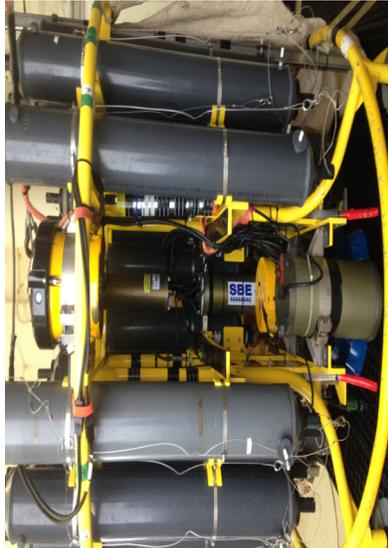
Photo 01: Instruments and battery pack on rosette. UVP is not mounted in this photo.
