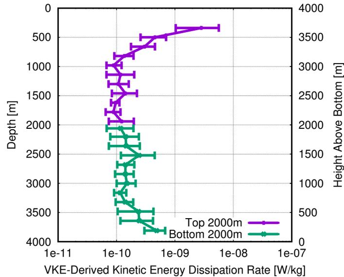
Figure 1: Section averaged profile of kinetic energy dissipation estimated from LADCP-derived vertical velocities using a finestructure parameterization method. Data from the top 2000 m are plotted against depth (left axis); data from the bottom 2000 m are plotted against height-above-bottom (right axis). Error bars are from bootstrapping.
