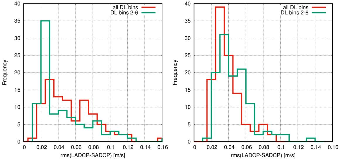
Figure 7: Histogram of  $rms$  LADCP-SADCP horizontal velocity differences from two cruises using the same WH150 ADCP. Left panel: 2015 P16 occupation before TRDI hardware upgrade. Right panel: 2016/17 P18 cruise, leg-1 data, after TRDI hardware upgrade.
