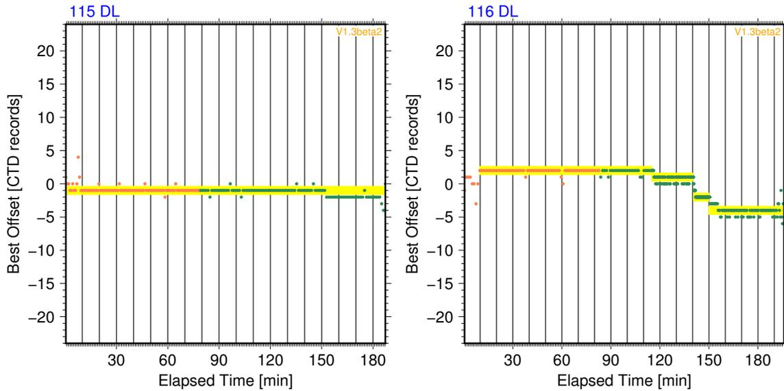
Figure 5: LADCP\_w time-lagging offsets from two example profiles. Left panel: Profile 115 without any dropped scans, resulting in a constant offset for the entire profile. Right panel: Profile 116 with several dropped scans, causing discrete steps in the offsets.
