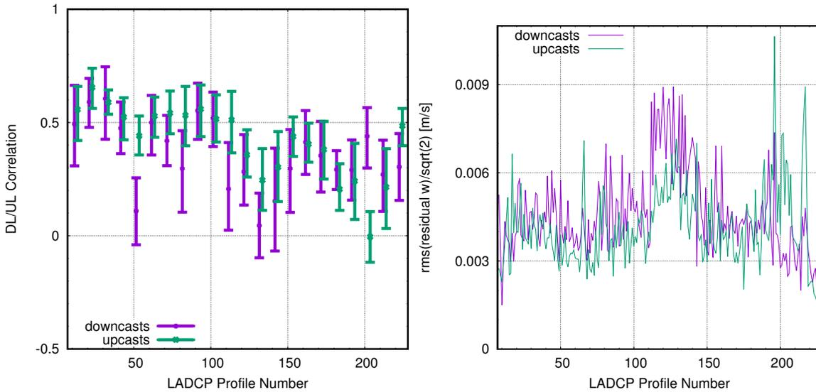
Figure 6: Vertical-velocity DL/UL correlations. Left panel: Correlation coefficient vs. profile number averaged in groups of 10 profiles, with error bars from bootstrapping; high values indicate good agreement. Right Panel: Corresponding regression residuals scaled by  $1/\sqrt{2}$ ; low values indicate good agreement.
