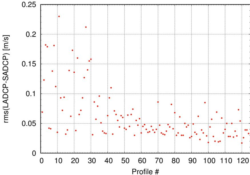
Figure 4: *rms* LADCP-SADCP horizontal velocity differences; low values indicate good agreement .
