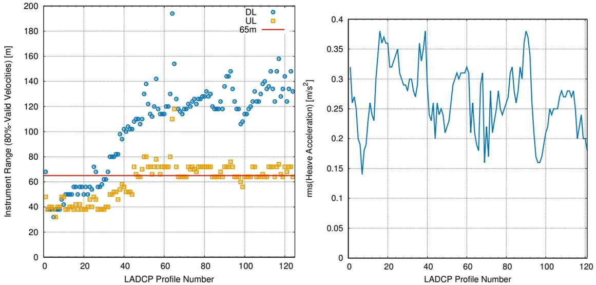
Figure 3: Left panel: Instrument range, with the red line indicating the minimum range (65 m) typically required for successful processing of full-depth LADCP profiles from a single 300 kHz TRDI Workhorse ADCP. Right panel: *rms* vertical acceleration due to vessel heave (sea state).
