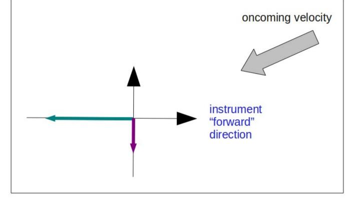
This is a top-down view of the measured horizontal velocity in ship coordinates.
