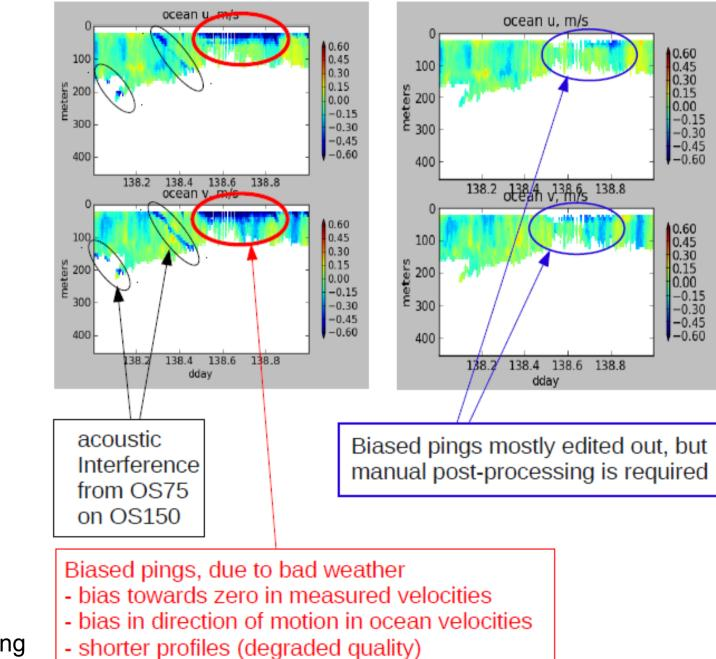
OS150 underway bias due to poor weather conditions
