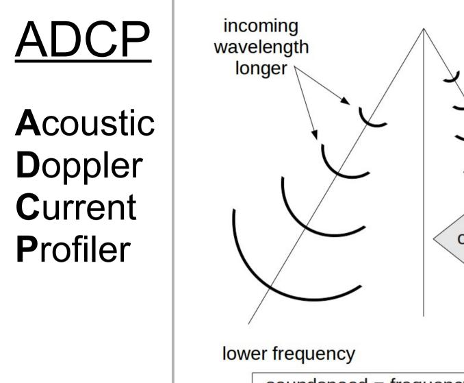
oncoming current higher frequency soundspeed = frequency X wavelength (ocean) (instrument)
