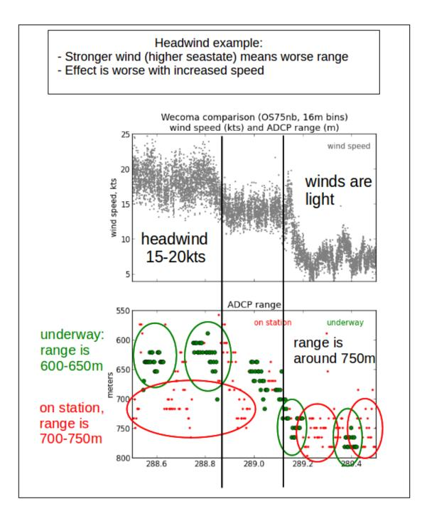
This plot shows windspeed (top panel) and ADCP range (bottom panel), with color-coded "on station" and "underway" periods. When the wind is high (at the beginning) the range decreases by 100m when the ship gets underway (green) compared to being on station (red). As the winds decrease, range increases to about 750m, regardless of whether the ship is on station or steaming.
