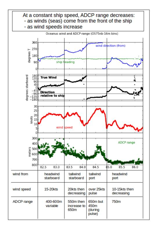
Range is decreased by the headwind more than the tailwind, but even with a tailwind, a pulse of wind at 84.5 is accompanied by a loss of range (150m-200m). This wind is shifty and may not accurately indicate the direction of the seas, but it is still clear: better data in low winds (750m range).
